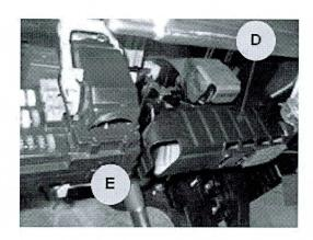
8. When removing the stop lamp switch in Entourage (EP) vehicles equipped with adjustable-height pedals, it may be required to loosen a mounting bracket to provide enough space to remove the stop lamp switch.
