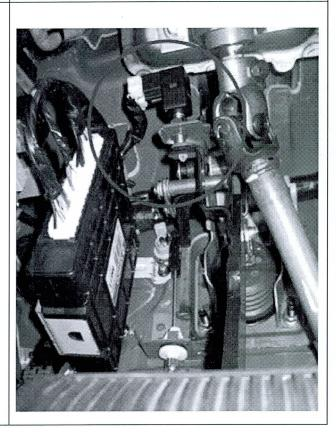
4. Loosen lock nut and remove the stop lamp switch from its mount. Disconnect the connector and remove the stop lamp switch from the vehicle.
