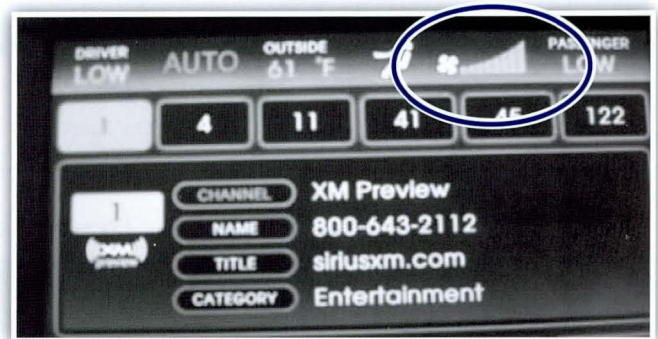
Fan speed after Voice Recognition / Bluetooth / Blue Link session (max speed – 8 bars)
