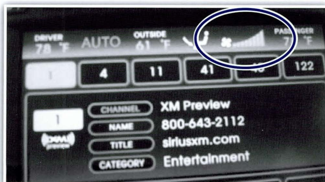
Fan speed before Voice Recognition / Bluetooth / Blue Link session (max speed – 8 bars)
