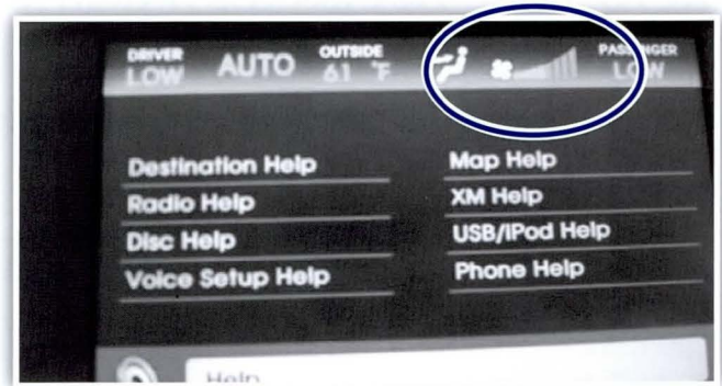
Fan speed during Voice Recognition / Bluetooth / Blue Link session (half speed – 4 bars)
