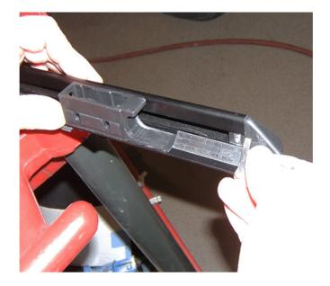
6. Reposition the pivot block 54.5 mm (2.15 in) from the end of the rail and re-secure the two set screws.
