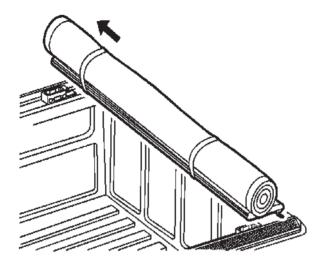
1. Remove the tonneau cover and the side rail(s) on the affected side. Refer to Soft Tonneau Cover Package Installation in SI.
