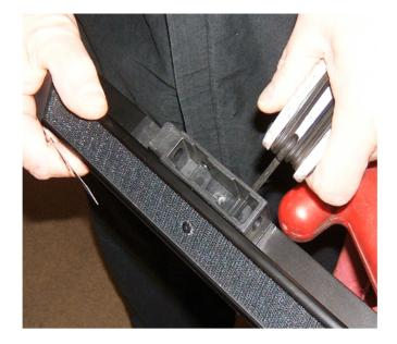
4. Loosen the two pivot block set screws securing the pivot block to the side channel of the rail assembly.
