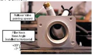
The fuel filler neck must be installed with proper orientation on the body. The neck should be installed with the roll-over valve pointing upward. The bottom edge of the neck mounting flange must be parallel to the ground. See photo for reference.
