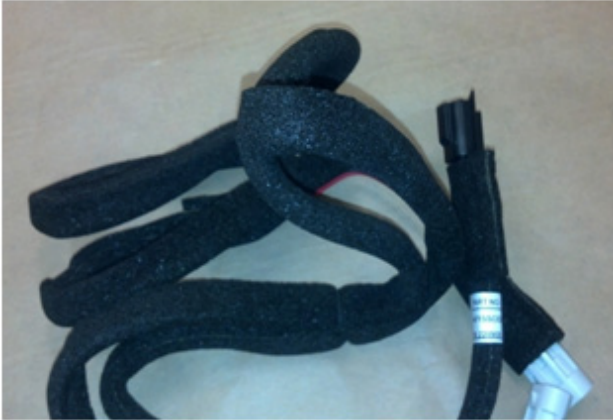
No in-line fuse installed
