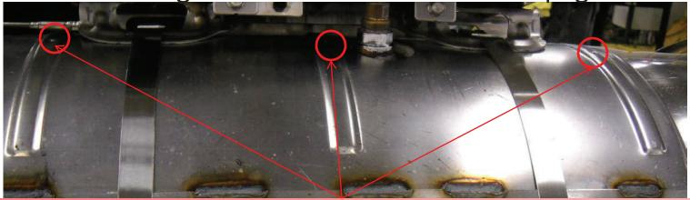
There are identifying "dimples" in the heat shield of a compatible SCR Catalyst
