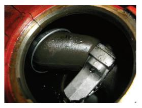
With a flashlight, review 4 digit casting on crankshaft. IF those digits are "22/12" or earlier, then compressor must be replaced. Otherwise, continue to next step. (Ex: The picture below has a crankshaft date code of "18/10" therefore, it would need replaced.)
