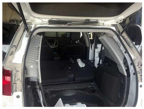
The cause of this condition may be that the dust/debris is working past the side door or liftgate sealing surfaces.
