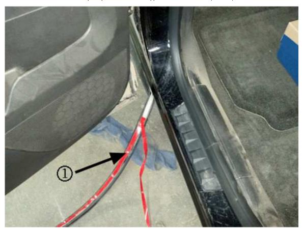
Note: The recommended size of the two-sided tape is approximately 1.5 mm (0.060 in) thick and 13 mm (0.500 in) wide.
