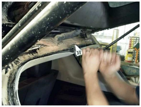
**3.5.** Using an adjustable wrench, or similar tool, carefully bend the pinch weld to a position perpendicular to the liftgate interface.
