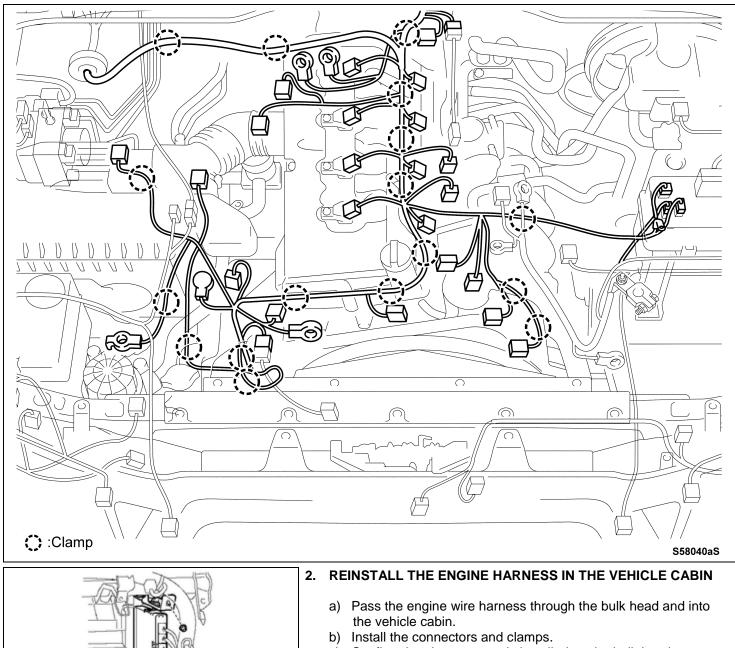
c) Confirm that the grommet is installed on the bulk head.
