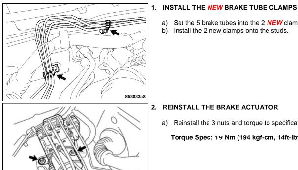
b) Install the 2 new clamps onto the studs.
