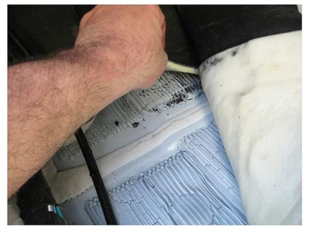
Inspect the vehicle for accumulated water or water spotting in the driver and passenger front footwell areas. Reposition the front carpet and inspect for
