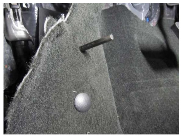
**10.** Install the push pins through each hole.
