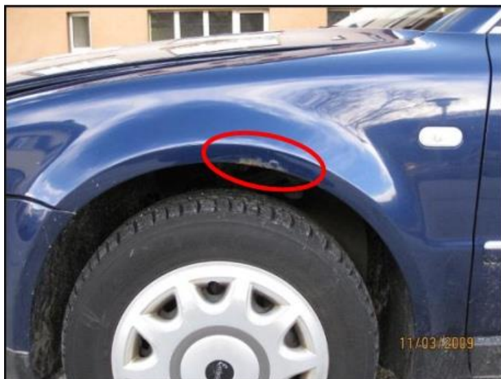
Figure 1 (corrosion on left wheel arch)
