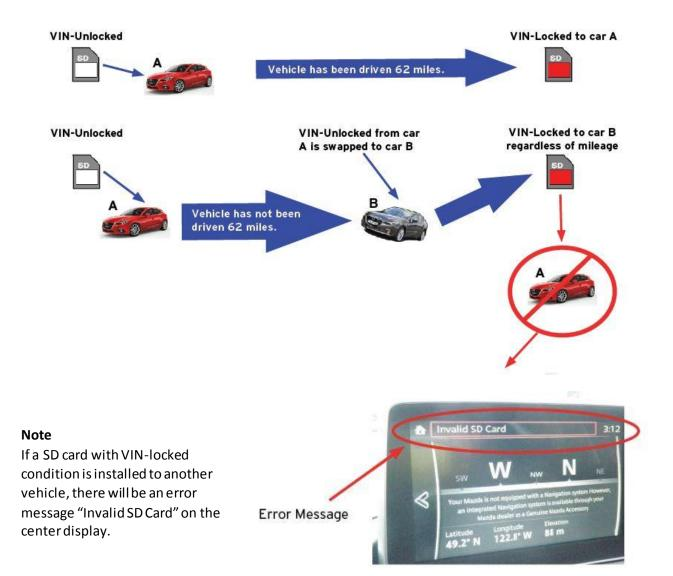
1. Error message may be displayed when SD Card is updated or replaced. The error message "Invalid SD Card" is displayed on the center display when there is a malfunction (as mentioned previously, unauthorized modification, hard core failure etc.) with the SD card.
