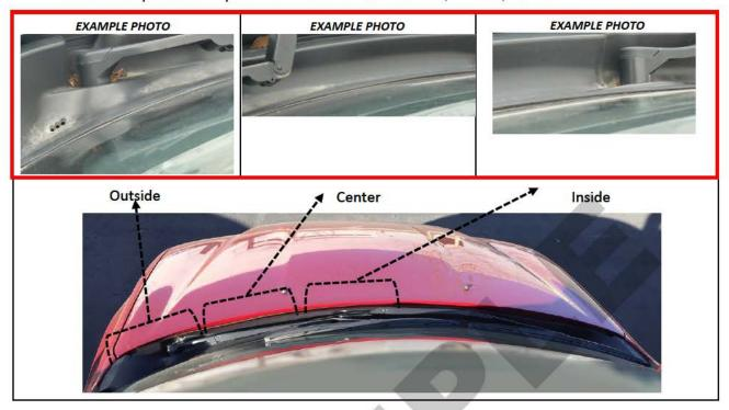
c) Measure gap between Deck Garnish and G s 10 cm intervals, starting at "G," as shown below.
