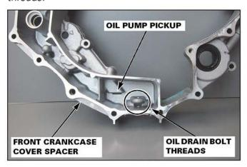
The best practice for repairing stripped drain bolt threads on these models is to replace the front crankcase cover spacer entirely, as it is virtually impossible to perform a reliable drain bolt thread repair on these models.
