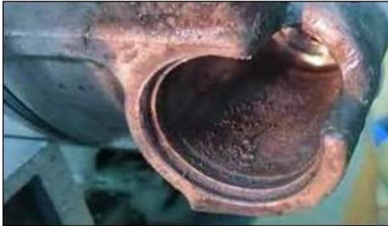
Figure 14. Corrosion in the N280 valve bore.
