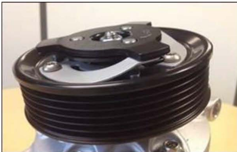
Figure 7b. Example of torque limiter over load protection still intact.
