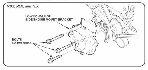
3. Using a die grinder with a 2-inch grinding disc, use the circular casting offset as a guide to grind the side engine mount bracket until the lip measures 2 mm in thickness.
