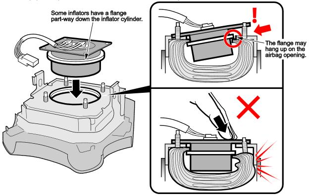
• Using a pair of pliers, gently pull up on each stud up while pushing the inflator module down until the airbag is properly seated within the airbag module.
