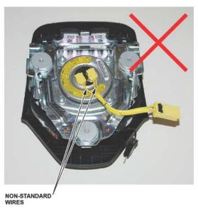
5. Remove the four horn plate mounting bolts, the mounting bolt felt washers, the horn plate, and remove the felt tape covering the lower two inflator locknuts. The felt washers and felt tape will not be reused.
