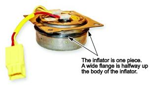
• Insert the airbag inflator into the opening. Do not force it into the airbag module.
