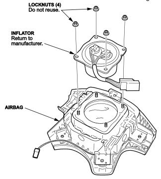
7. Use shop air to clean any debris that may be on the inflator, then remove the inflator from the airbag.
