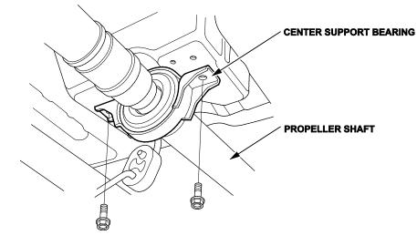
7. Install the new propeller shaft by aligning the factory reference marks on the No. 2 propeller shaft to the rear differential companion flange as shown below. Then install new flange bolts and torque them to **72 N·m (53 lb-ft)**.
