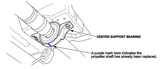
3. Remove the propeller shaft protector.
