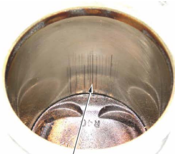
Light scratches are not abnormal. Ensure a fingernail or pencil "catches" on the scratches before replacing the block.
