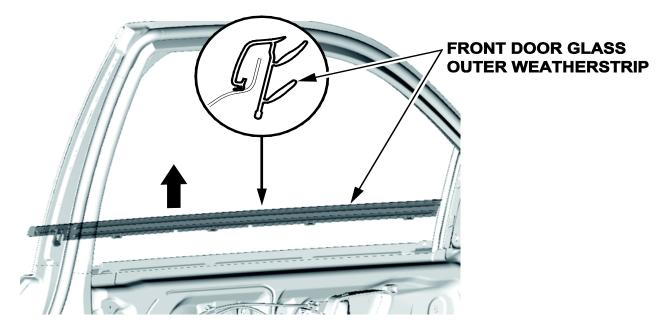
6. Lightly pull away the door weatherstrip from the top corner just enough to remove the screw on the end of the chrome molding. Lightly pull away the top end of the chrome molding, detach the clip, then remove the door sash trim.
