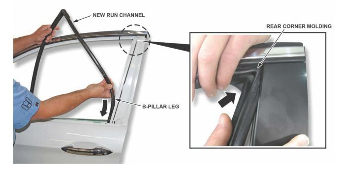
3. After setting the rear corner molding, begin setting the run channel in the window frame toward the front sash. Now slide the A-pillar leg of the run channel down between the glass and the front steel channel.
