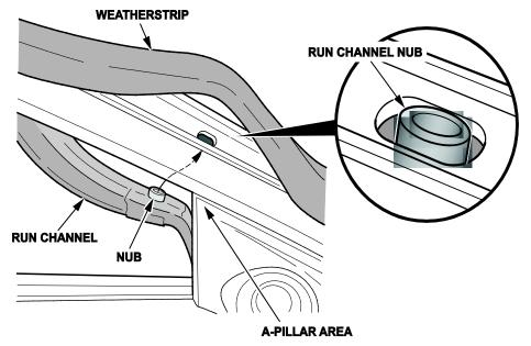
7. Set the A-pillar leg of the run channel down into the door. Set the outside attachment first, then set the inside attachment of the run channel.
