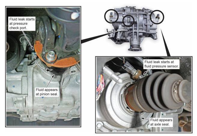
Before considering rear differential replacement, be sure to check those items carefully. The repair could be as easy as tightening or replacing the fluid pressure sensor or tightening the fluid pressure check port.
