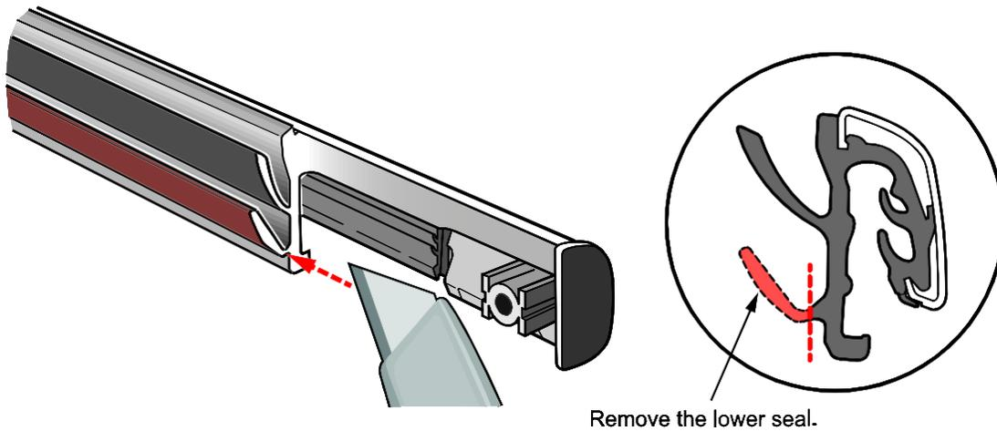
6. Reinstall the outer door glass weatherstrip.
