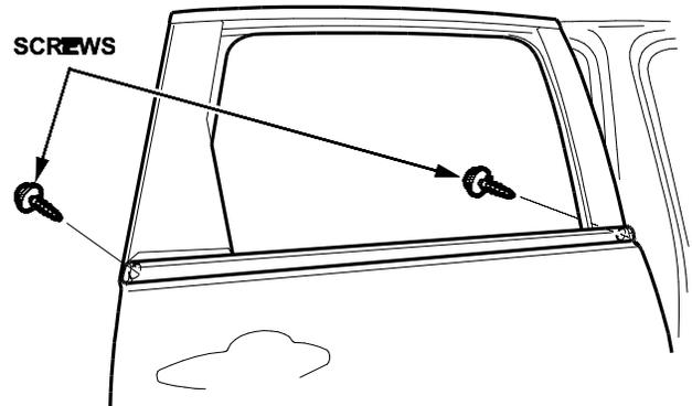
3. Starting at the rear, pull up on the door glass outer weatherstrip at each area where the inner molding catches the inside edge of the window slot.
