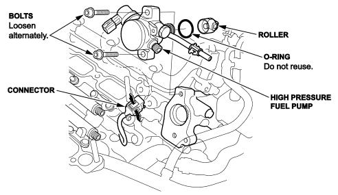
9. Remove the bolts by loosening them alternately, then remove the high pressure fuel pump and the roller.
