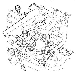
27. Install the intake base and intake manifold.
