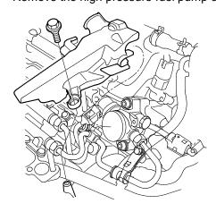
5. Remove the quick-connect fitting cover.
