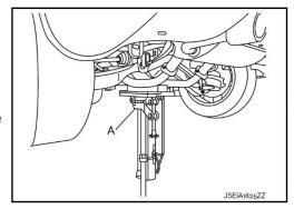
3. Lift the vehicle and move the tires ① up and down by hand to check if the ball joint has a backlash. If it has a backlash, replace trans-verse link.
