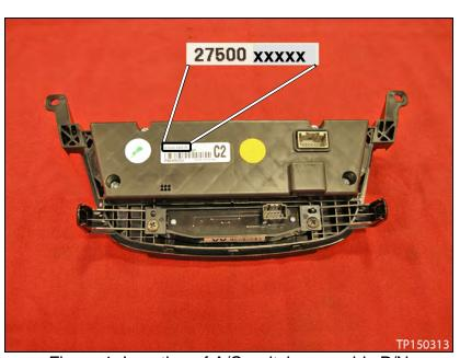
Figure 1: Location of A/C switch assembly P/N
