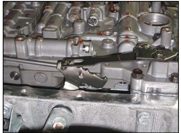
Figure 2. Detent Spring in Place on Manual Shift Lever (Transmission Oil Pan Removed for Clarity)
