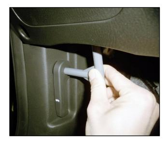
2. While applying slight inward pressure to the end of the SST, use a plastic prying tool to remove the hood release lever.
