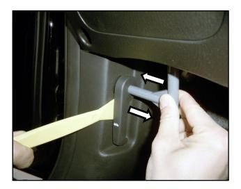
3. To reinstall, place the hood release lever on the pivot point and gently snap it in place.
