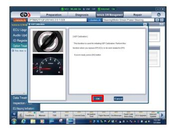
9. Start the engine and center the steering wheel. Then, click on **OK**.
