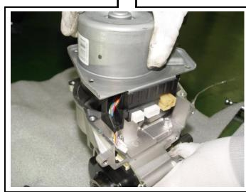
Remove the original flexible coupling
