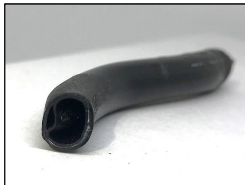
Restricted Fuel Line
