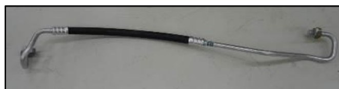
A/C Discharge Hose
