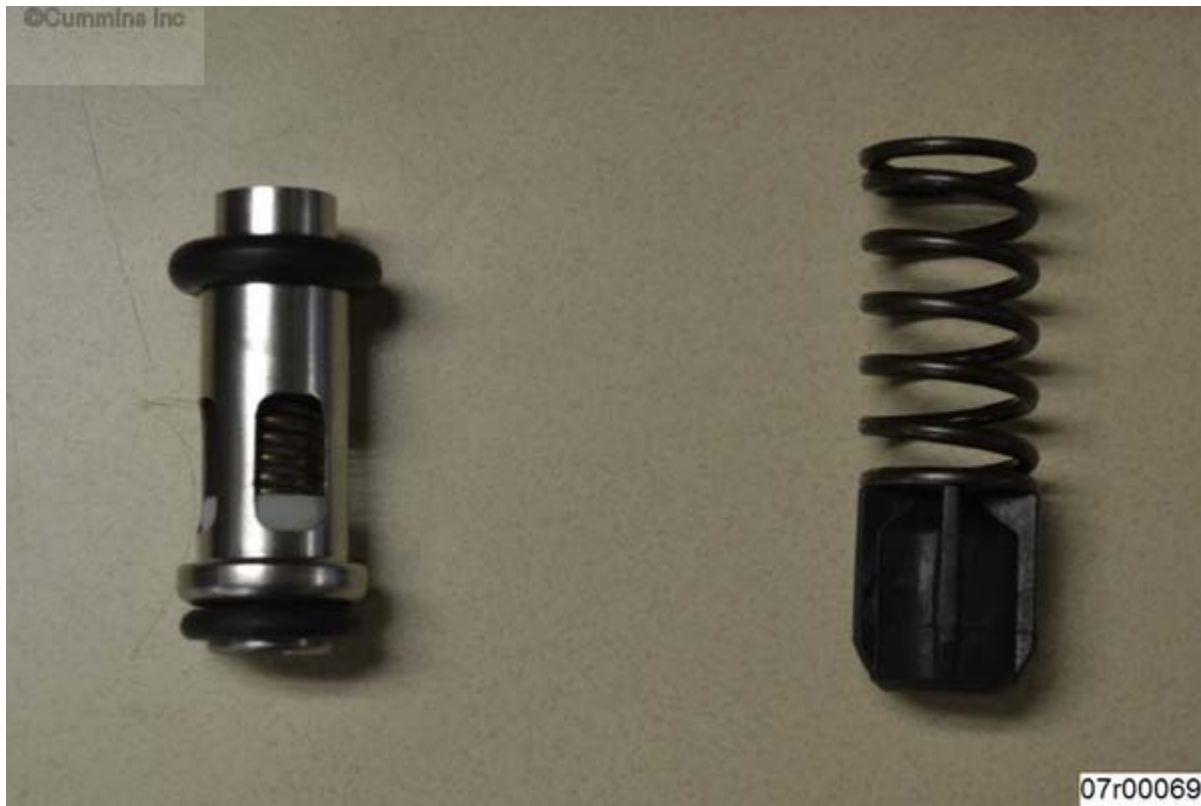
Figure 3, Left: New Single Piece Cartridge Style Bypass Valve. Right: Obsolete Spring and Bypass Valve.
