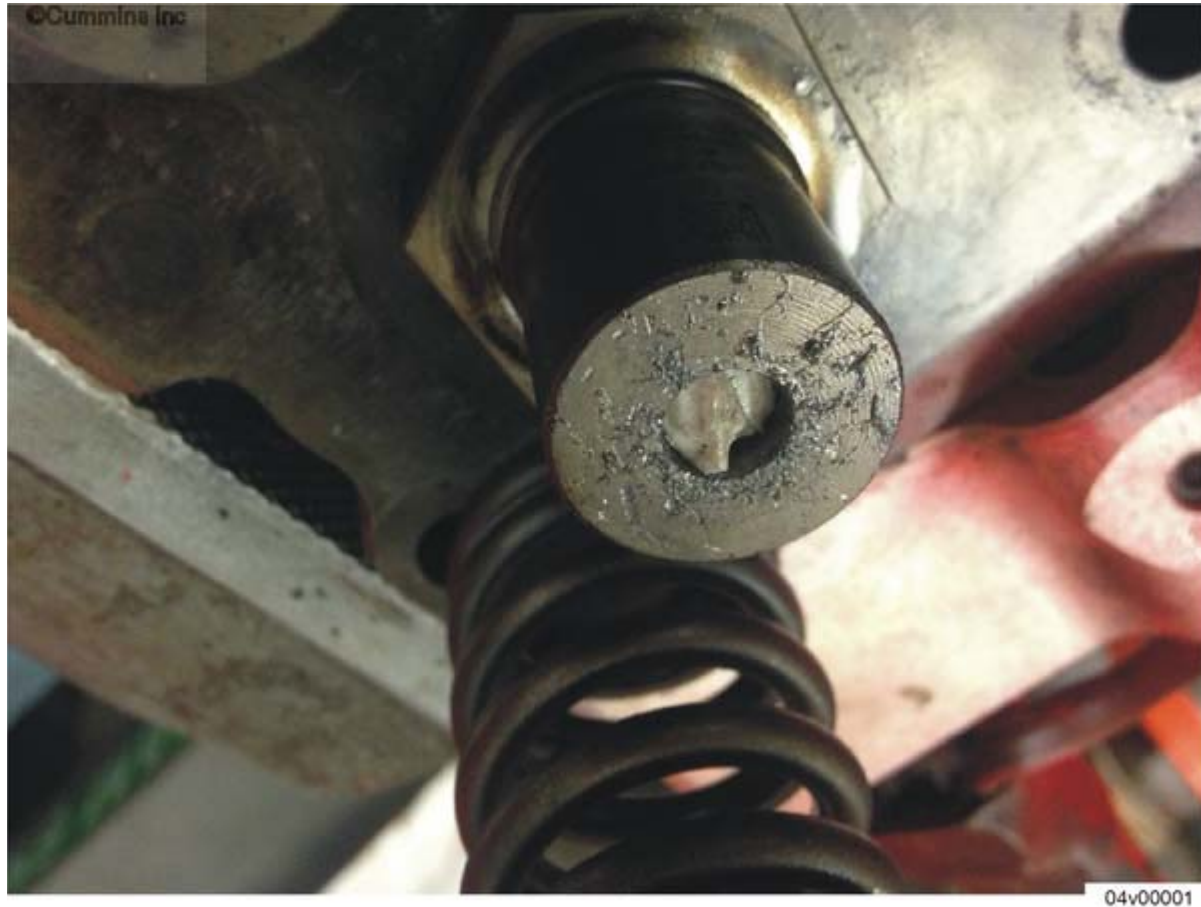
Figure 1, Fractured Fuel Pump Ceramic Pumping Plunger on CM2250 Engines.
