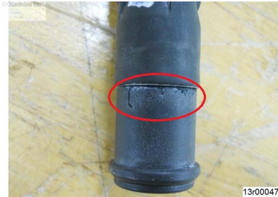
Figure 2, Example of Signs of Arching on Ignition Coil.
