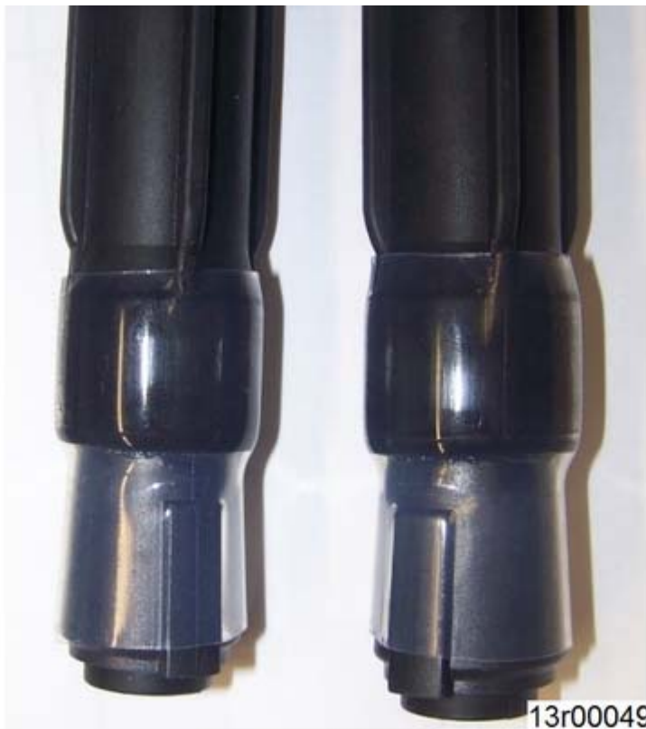
Figure 1, Example of Dielectric Heat Shrink Installed on Ignition Coil Extension.
