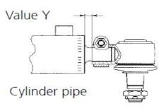
Value X (piston rod): Master cylinder: max. 13 mm (for 8346 974 163:max. 31.5 mm)
