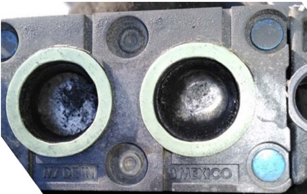
Figure 1 Example of water frozen on the sensor membrane
