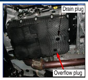
ATF TEMPERATURE = 122~140°F (50~60°C) SHIFT LEVER IN "N" AND ENGINE RUNNING
