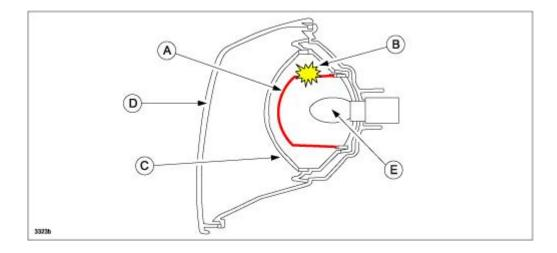
Customers having this concern should have both rear combination lights replaced with modified ones(red inner cap (A) is eliminated and red inner lens (B) is used).
