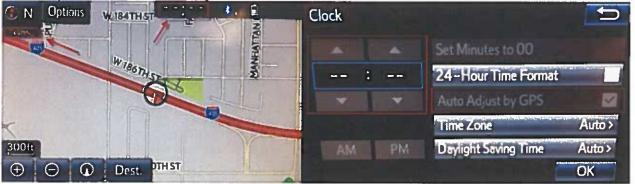
If the GPS icon on the navigation screen\* is grey but has no slash through it and the clock shows dashes, move the vehicle outside to get a GPS signal.
