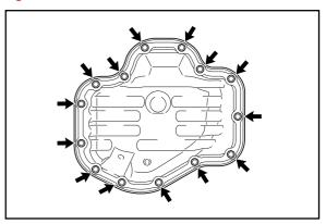
(2) Insert the blade of the Gasket Seal Cutter Figure 3. between the crankcase and oil pan. Cut through the sealer and remove the oil pan.
