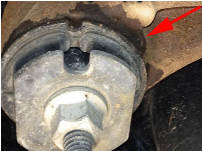
There is slight staining around the mount, but there are no droplets formed and fluid has not dripped onto other components.
