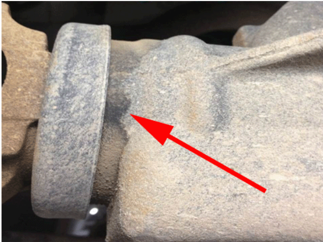
You can see the darker area where fluid has attracted dirt. There are no droplets at the bottom of the seal area.
