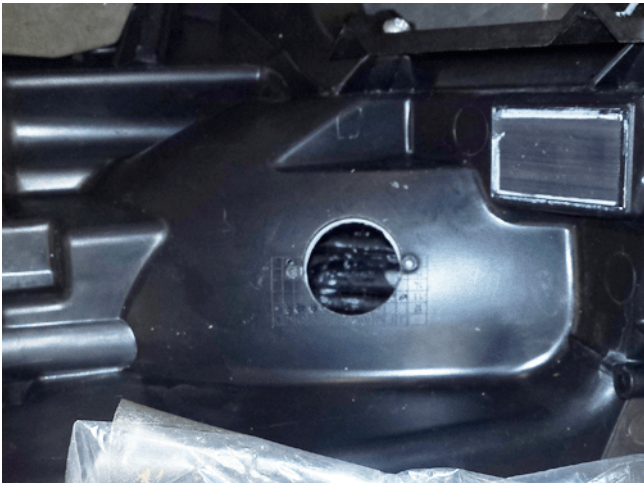
This housing shows a hole which was drilled in the lamp to accept an accessory modification.
