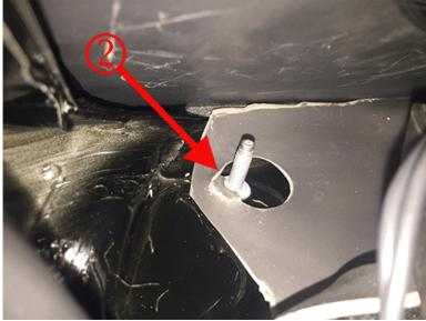
2. Inspect the B+ battery cable at the starter solenoid for shorting out on the starter heat shield, as shown below. If the battery cable is shorting on the starter heat shield, replace the B+ battery cable and starter heat shield. After installing the new starter heat shield and B+ battery cable, ensure there is adequate clearance so it will no longer short out.
