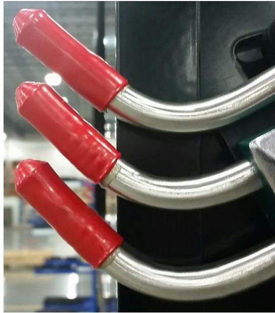
Figure 5 Correctly installed vent caps.
