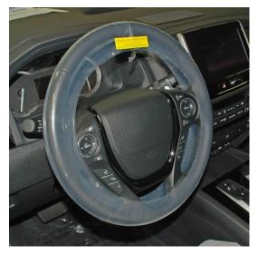
The easiest way to remove it during TQI is to grab the covering with both hands near the top of the steering wheel and pull it **toward** you, like you see here. The covering comes right off.
