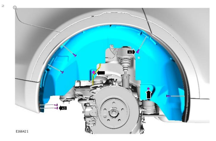
Remove the rear right splash shield.
