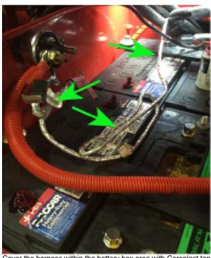
4. Cover the harness within the battery box area with Coroplast tape, using a ¼ in. overlap to ensure that no aluminum is exposed.
