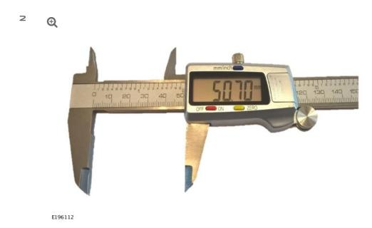
Set a vernier caliper to 50.70mm.
