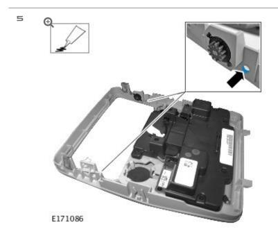
Apply Nyogel® 774L (or equivalent) into the hinge pin holes.
