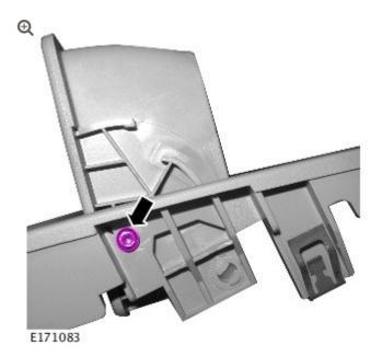
Remove and discard the retaining screw on the side of the sunglasses holder.
